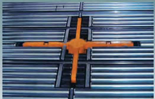
Integrated Lift and Turn Mechanism
